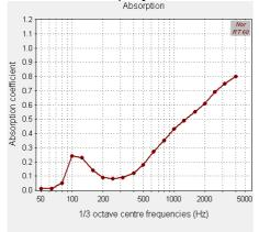
Name: 12mm polyester board on Plasterboard wall (combined absorption)
